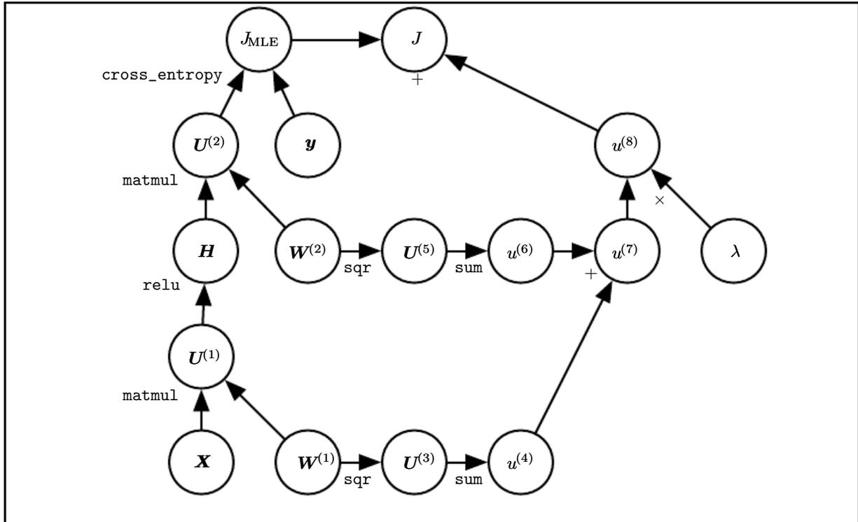
Figure 6.11: The computational graph used to compute the cost used to train our example of a single-layer MLP using the cross-entropy loss and weight decay.
